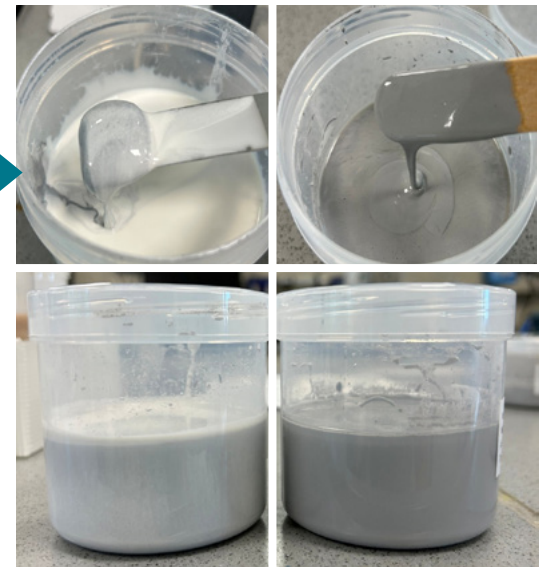
Borchi® Gel A LA No separation or sedimentation after 4 weeks
